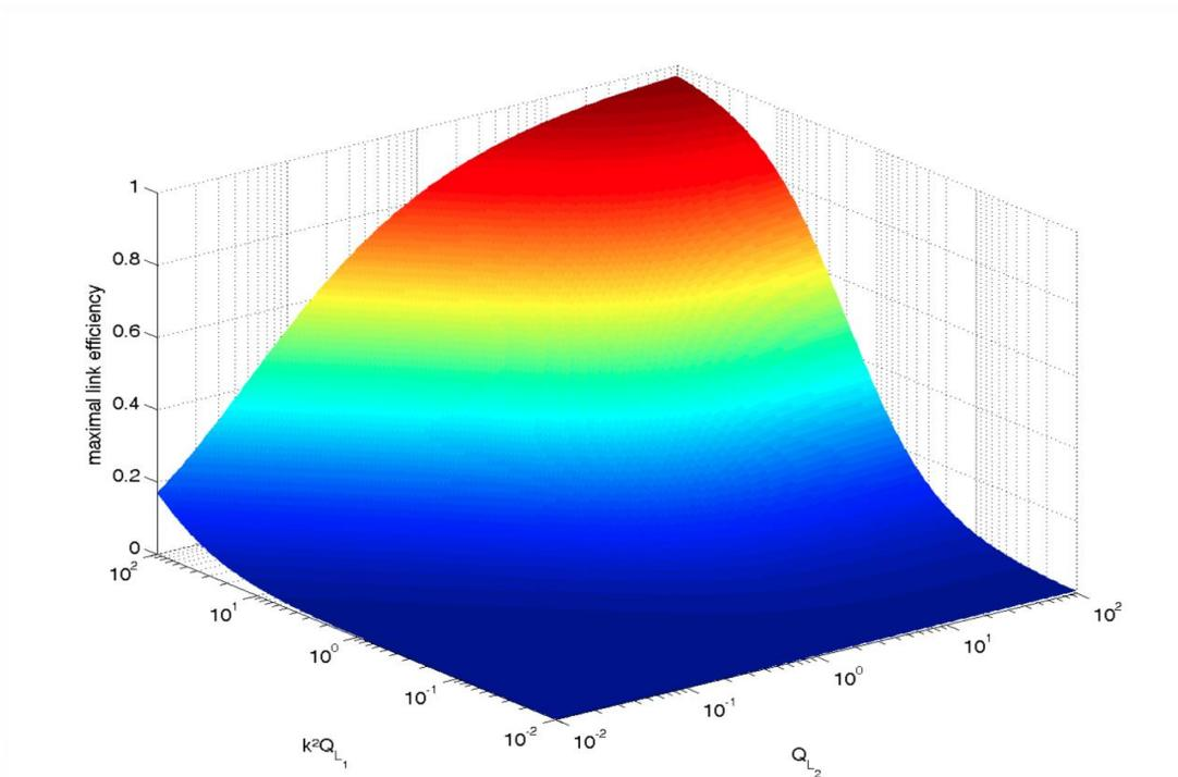
Figure 10 Link efficiency vs. coil quality factor
