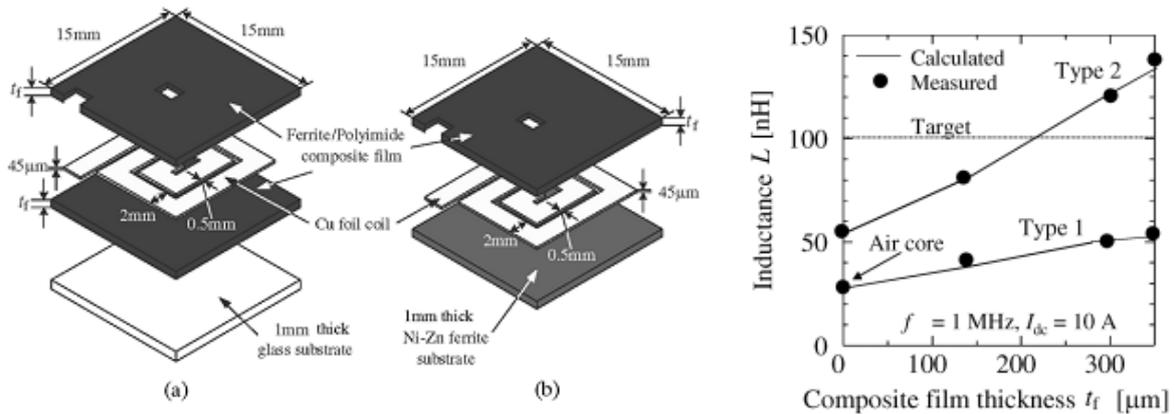
Figure 39 Integration of magnetic sheets into planar substrate
