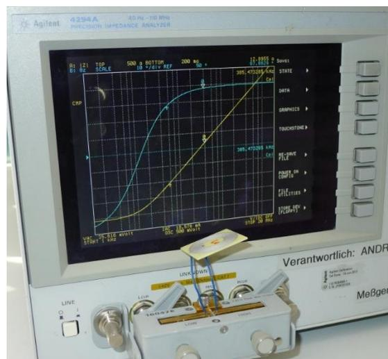
**Figure 34 Measurement set-up for characterizing the electrical characteristics of the coils**
