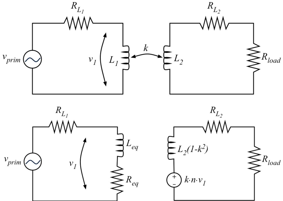
Figure 9 Equivalent circuit of non-resonant magnetic link
