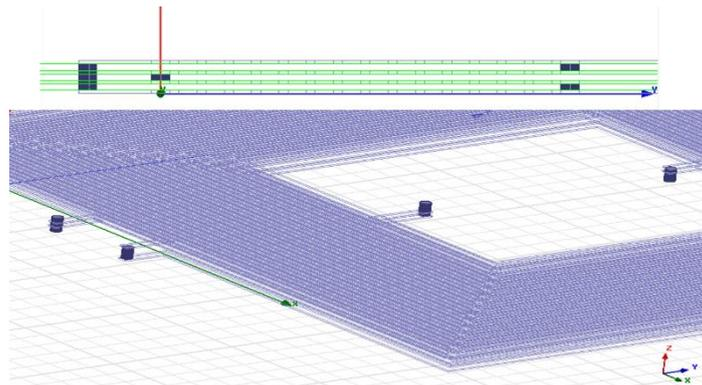
**Figure 24 Thru hole vs blind vias - simulation set-up**
