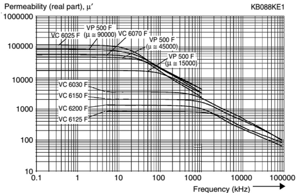
**Figure 38 Frequency Dependency of Vitroperm material**
