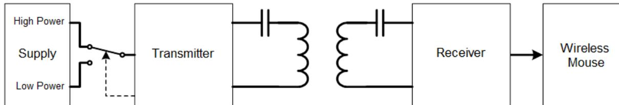
**Figure 53** Block diagram of wireless mouse test case
