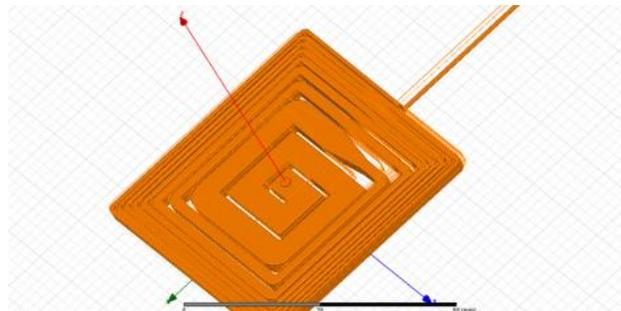
Figure 22 Simulation model of a staggered coil
