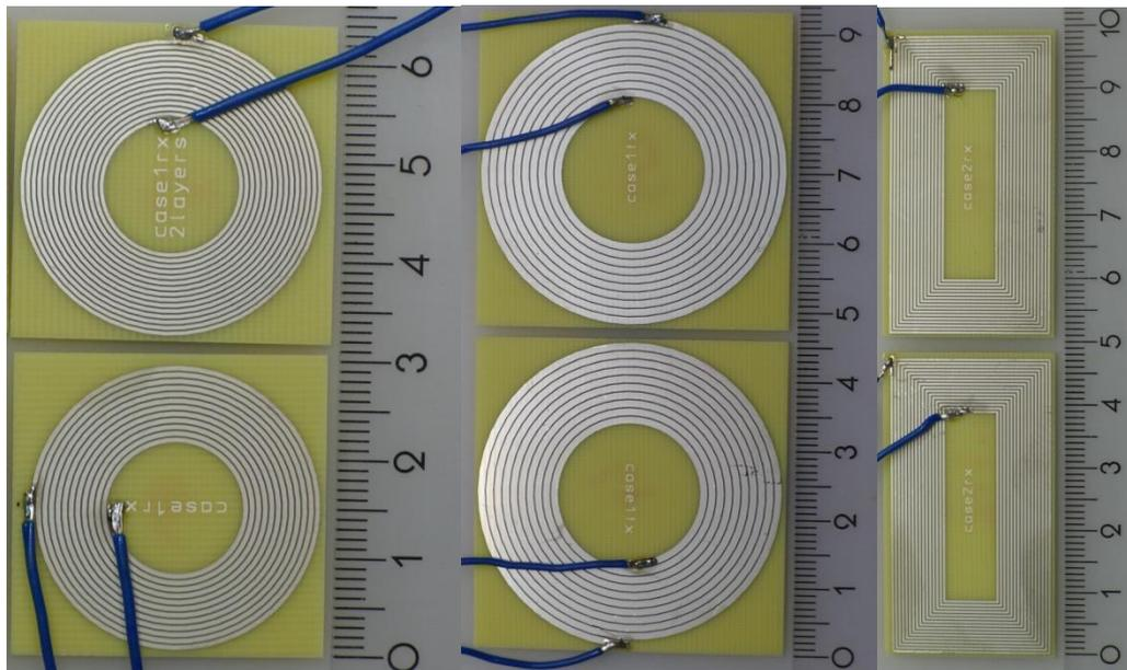
**Figure 33 Test samples for transformer coils**
