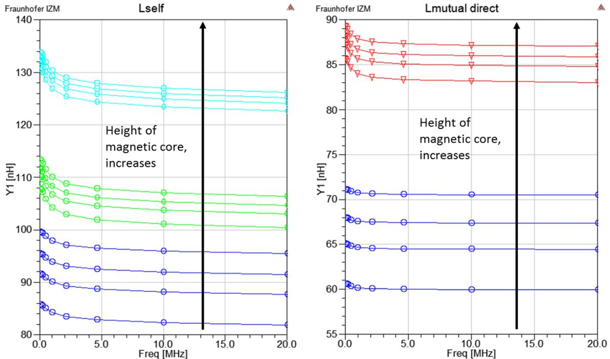
Figure 48 Influence of magnetic core height on trace inductance
