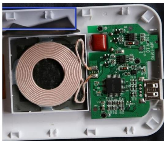
**Figure 12 Qi compatible charging station**
