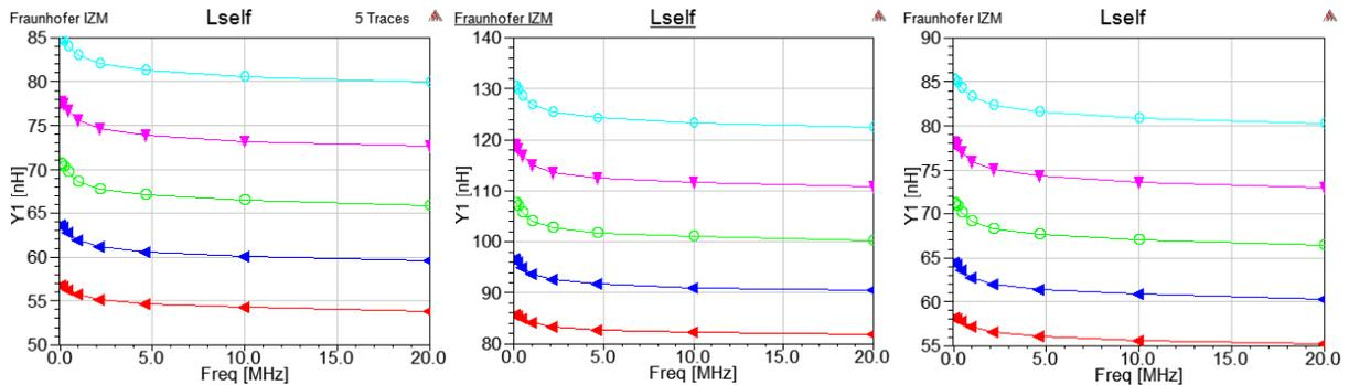
Figure 46 Influence of ferrite placement on self-inductance
