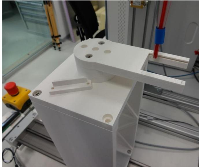
**Figure 32 Set-up for measuring the magnetic field and the coupling factor**
