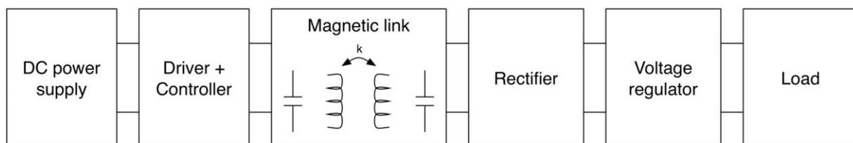
**Figure 8 System-Level model of wireless charging system**
