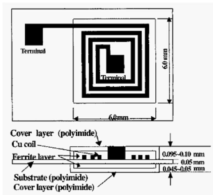
Figure 41 Substrate integrated coils with electrodeposited ferrite layer
