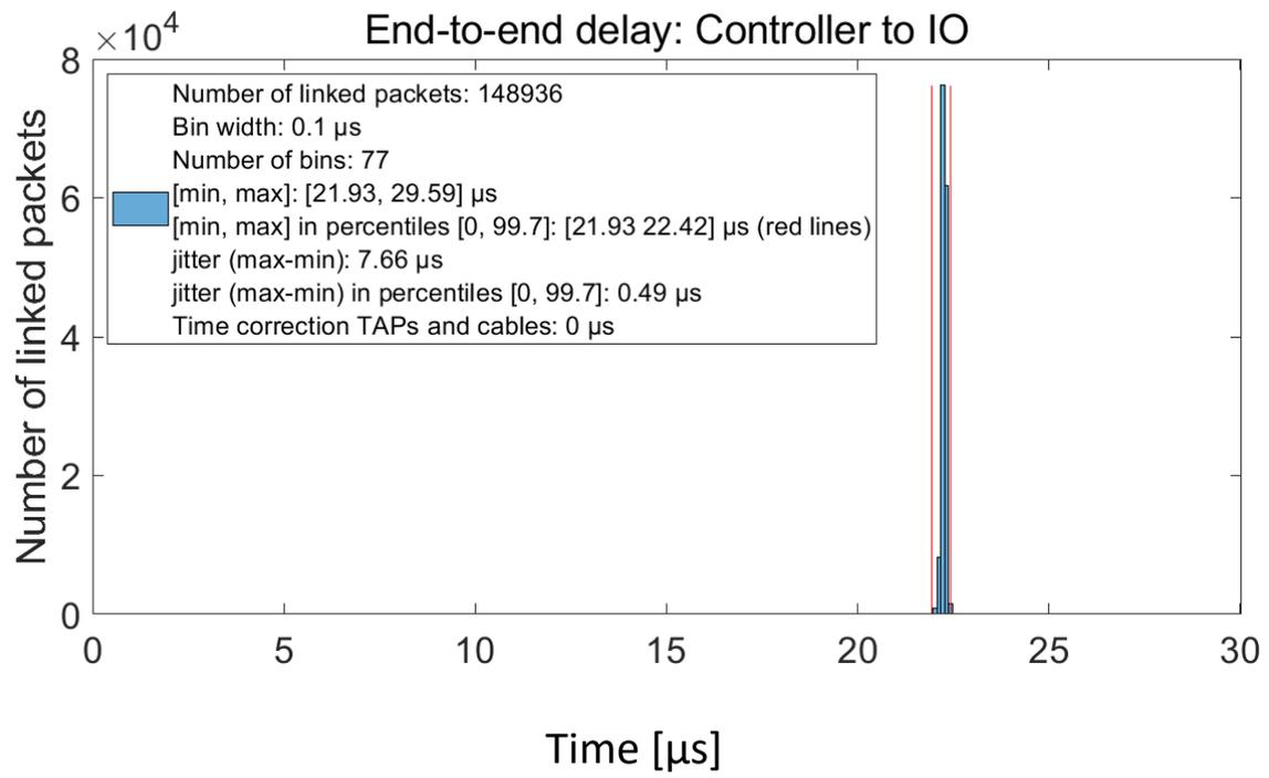
Figure 123: Relyum and NXP, 1000BASE-T, without preemption, without BE traffic
