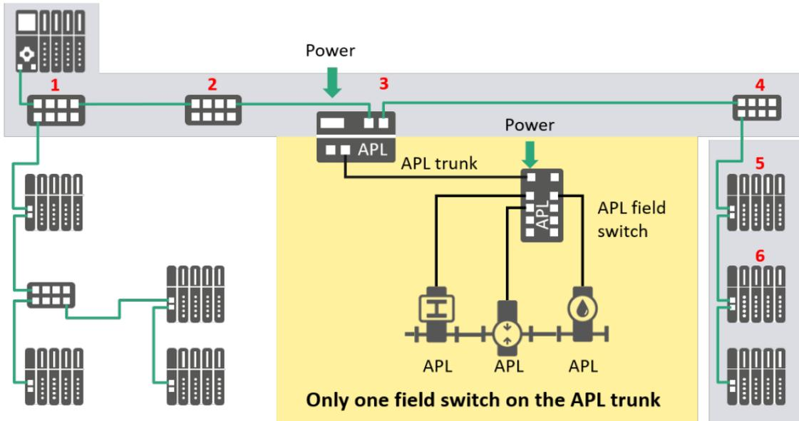
Figure 83: Line depth with APL trunk<sup>8</sup>
