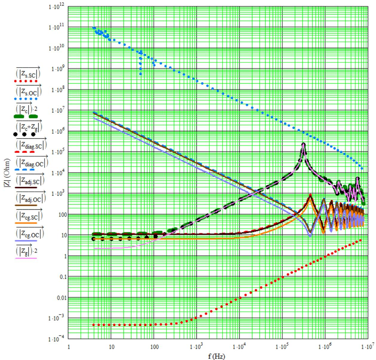
Figure 48. Source ( $Z_s$ ), calibrated wire ( $Z_c$ ,  $Z_g$ ) and 2cTL ( $Z_{diag}$ ,  $Z_{adj}$ ,  $Z_{cg}$ )  $|Z|$  (y-axis) over frequency (x-axis) for the solid wires cable. The  $|Z_s|$  curves are well distanced from the cables  $|Z|$ , ensuring a better measurement calibration.
