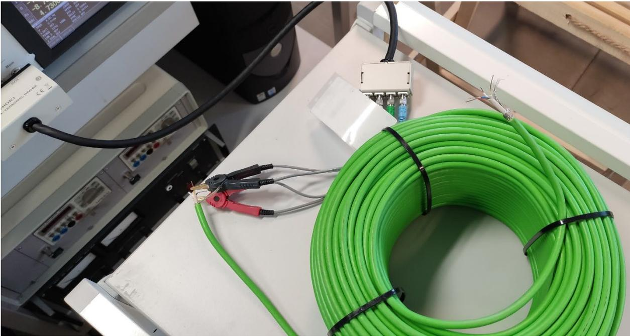
*Figure 46. Rolled cable under test (OC measurement).*
