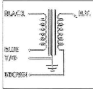
Figure 185: Connections of ignition transformer
