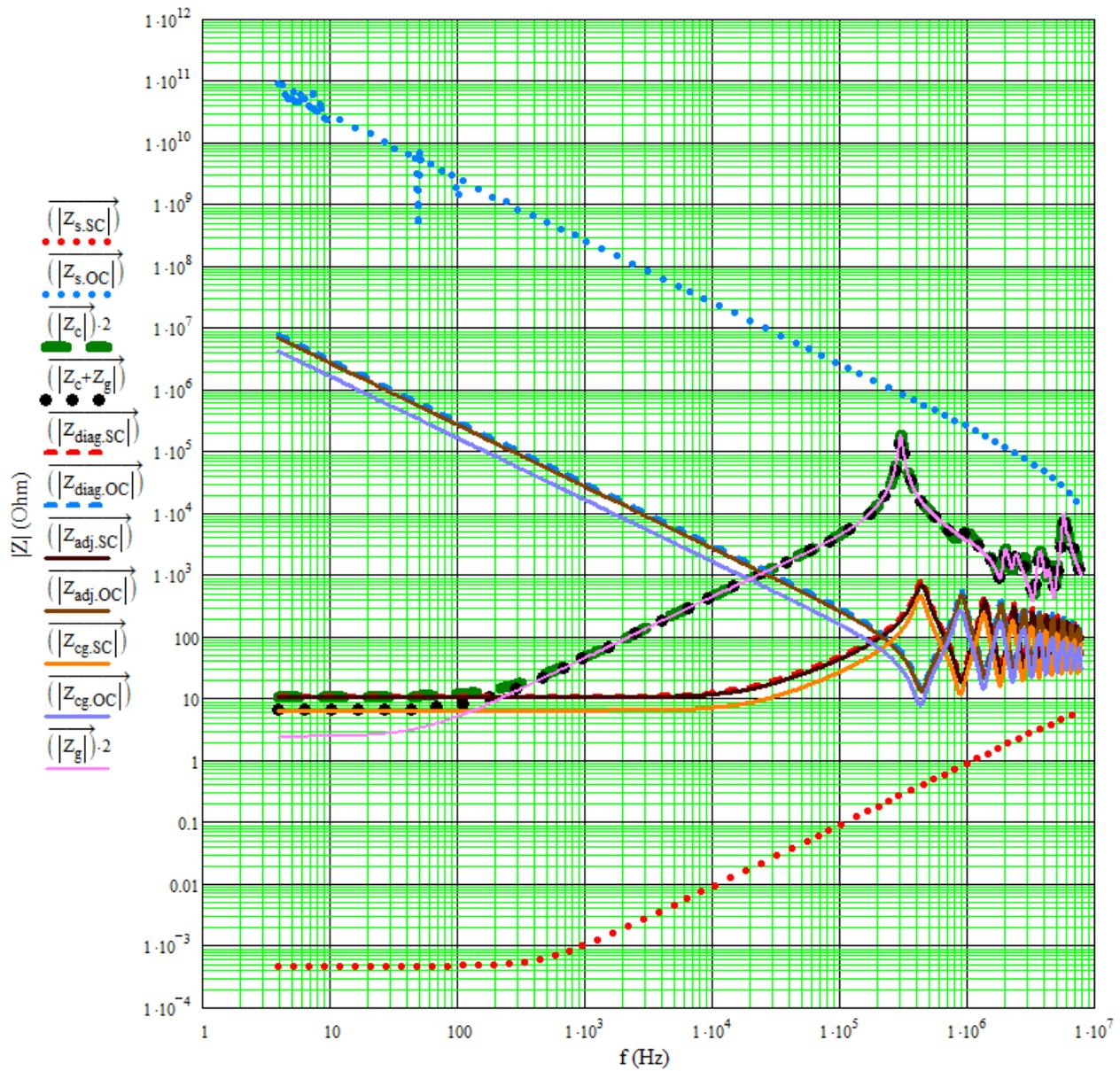
Figure 47. Source ( $Z_s$ ), calibrated wire ( $Z_c$ ,  $Z_g$ ) and 2cTL ( $Z_{diag}$ ,  $Z_{adj}$ ,  $Z_{cg}$ )  $|Z|$  (y-axis) over frequency (x-axis) for the stranded wires cable. The  $|Z_s|$  curves are well distanced from the cables  $|Z|$ , ensuring a better measurement and calibration.
