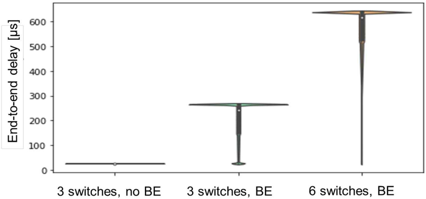
Figure 80: End-to-end delay on 100BASE-TX (35 Mbps BE)
