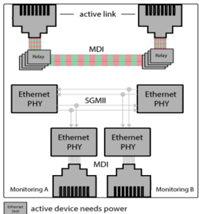
Figure 100: Schematic representation of a 1000BASE-T TAP in powered and unpowered state
