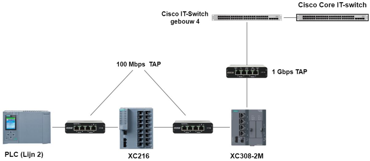
Figure 203: Schematic simplified overview of the placement of the TAPs
