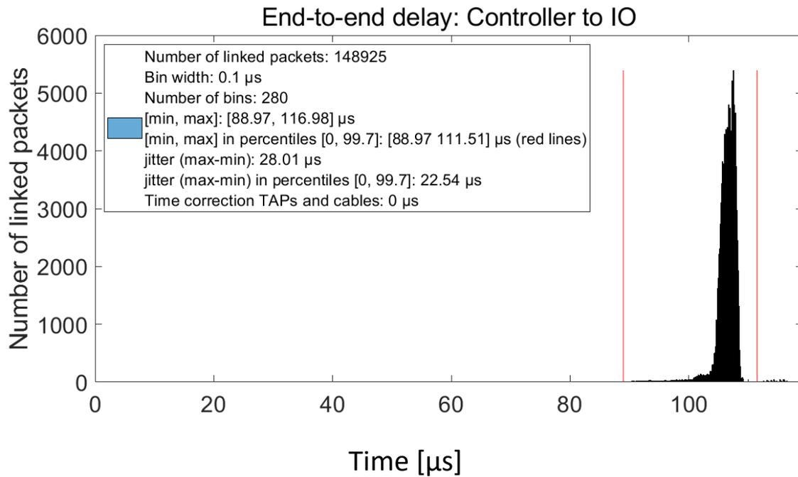
Figure 127: Phoenix Contact and NXP, 1000BASE-T, without preemption, with BE traffic
