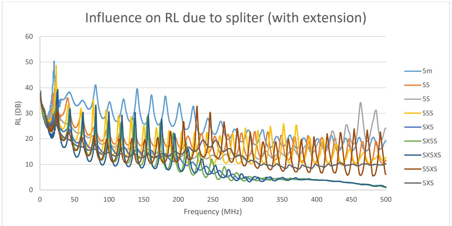
Figure 67: Influence on RL due to spliter (with extension)
