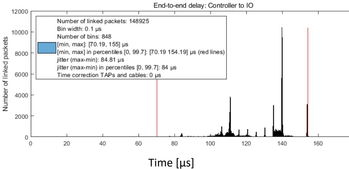
Figure 121: Relyum and NXP, 100BASE-TX, with preemption, with BE traffic
