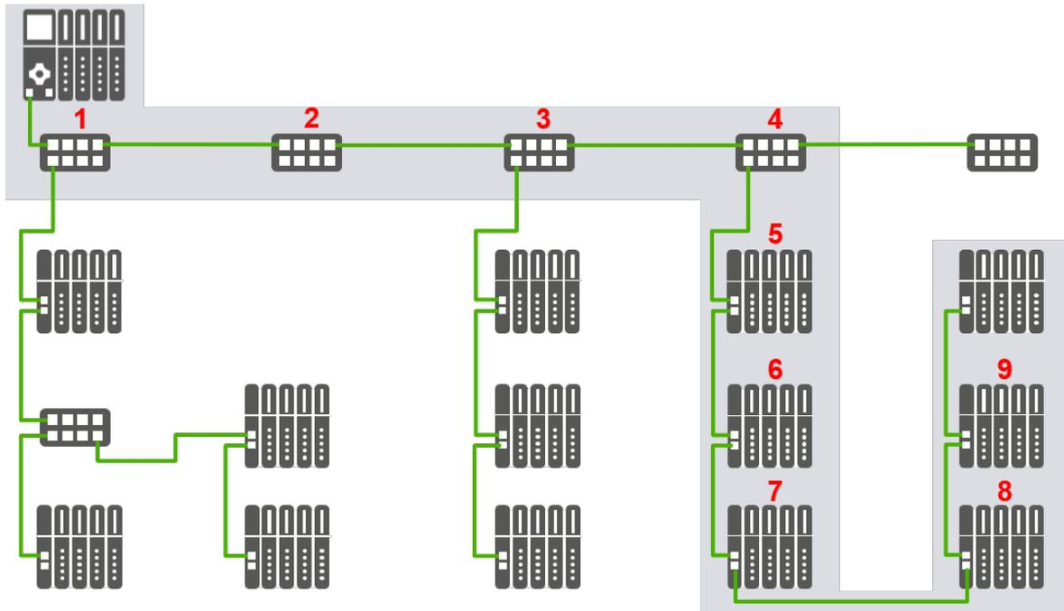
Figure 77: Line depth example<sup>6</sup>
