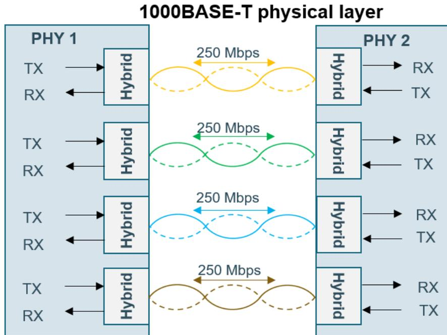
Figure 94: Schematic representation of 1000BASE-T communication
