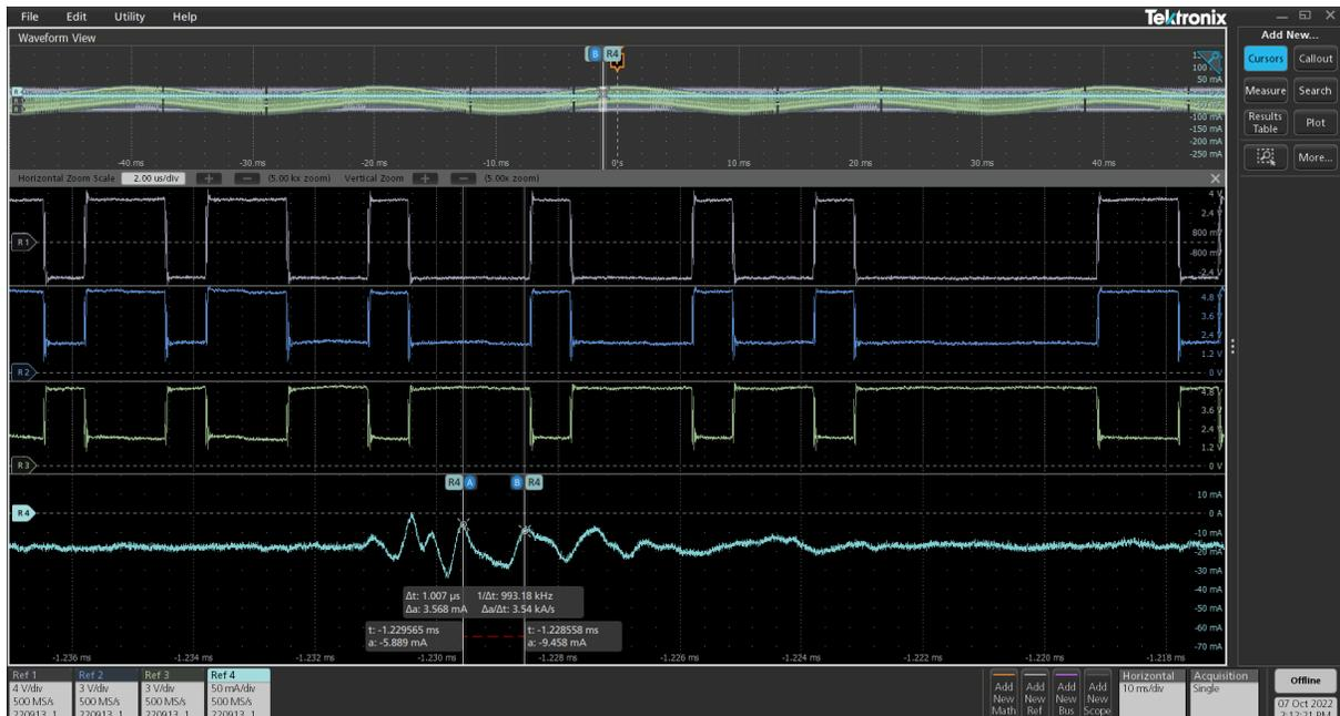
Figure 153: Zero measurement with loose capacitor no burner pulses (segment A2825) (5)
