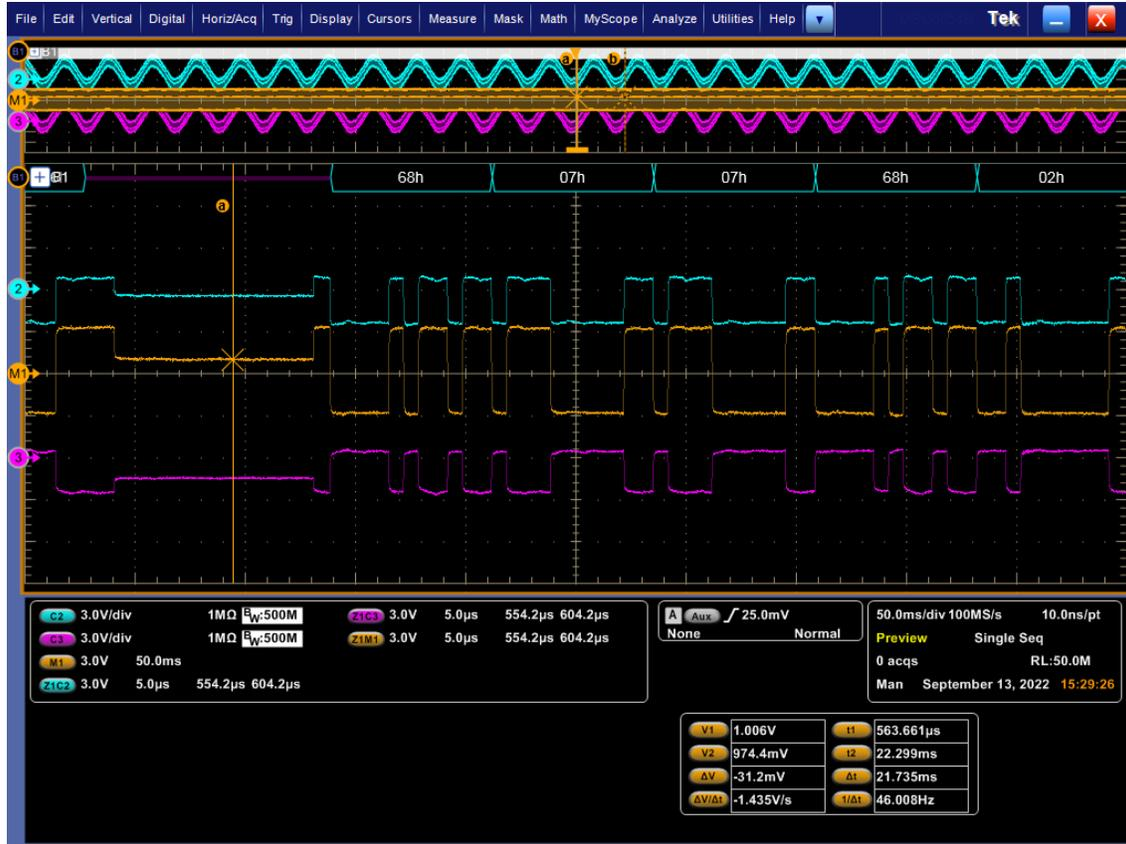
Figure 189: Measurement at station 61 (last slave of a segment) (3)
