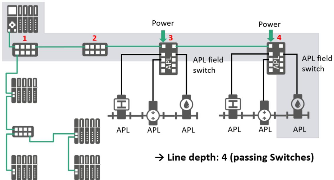
Figure 82: Line depth with APL Field-switches connected to 100 Mbit/s network<sup>8</sup>
