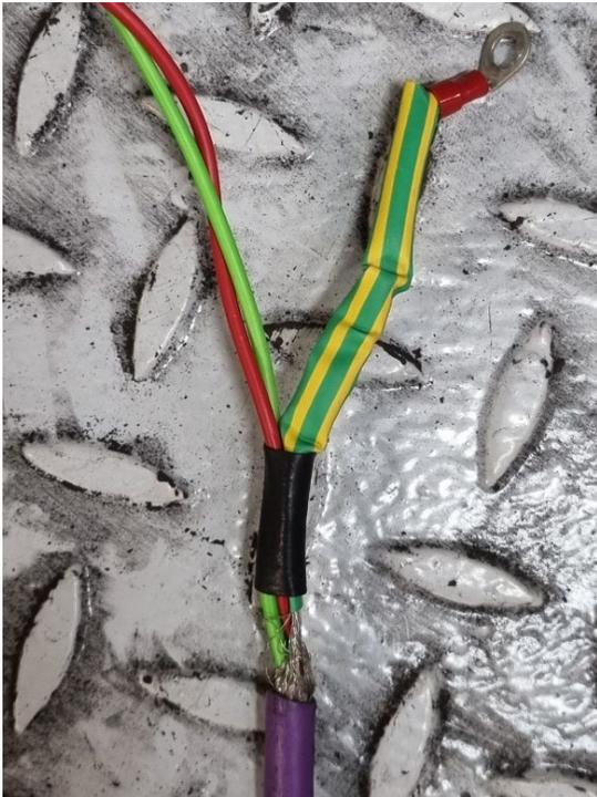
Figure 147: Detail of the PROFIBUS cable (2)
