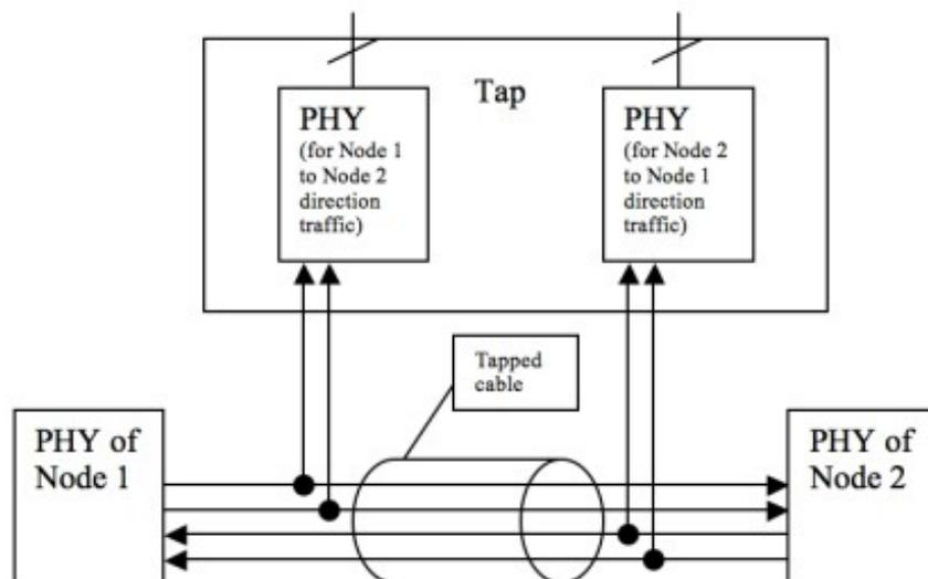
Figure 99: Schematic representation of a 100BASE-TX TAP
