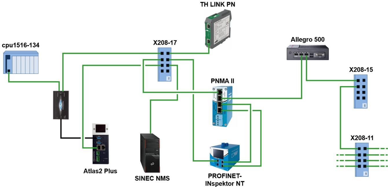
Figure 205: Backbone of the test network
