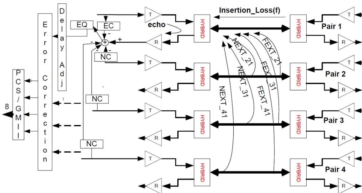
Figure 96: DSP-based adaptive filtering<sup>10</sup>
