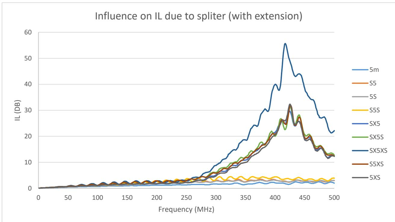
Figure 66: Influence on IL due to splitter (with extension)
