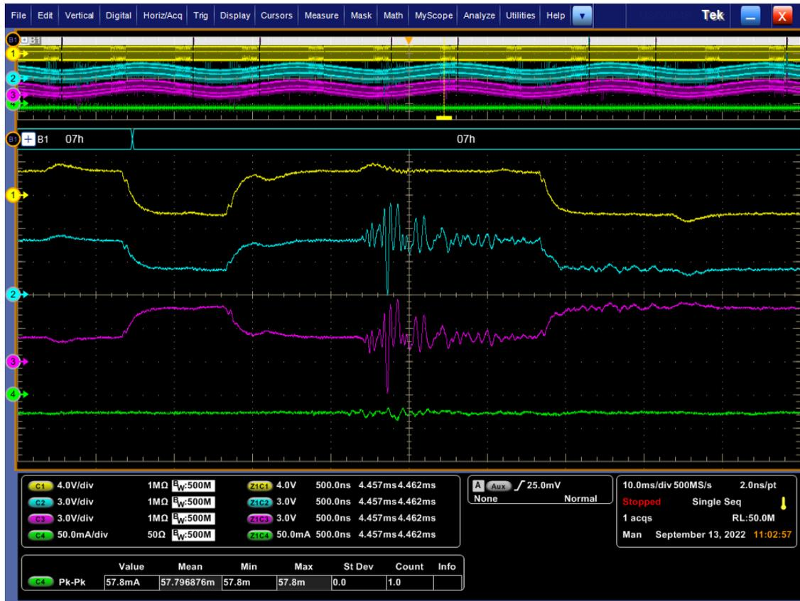
Figure 155: Ignitions with separate capacitor (segment A2825) (2)
