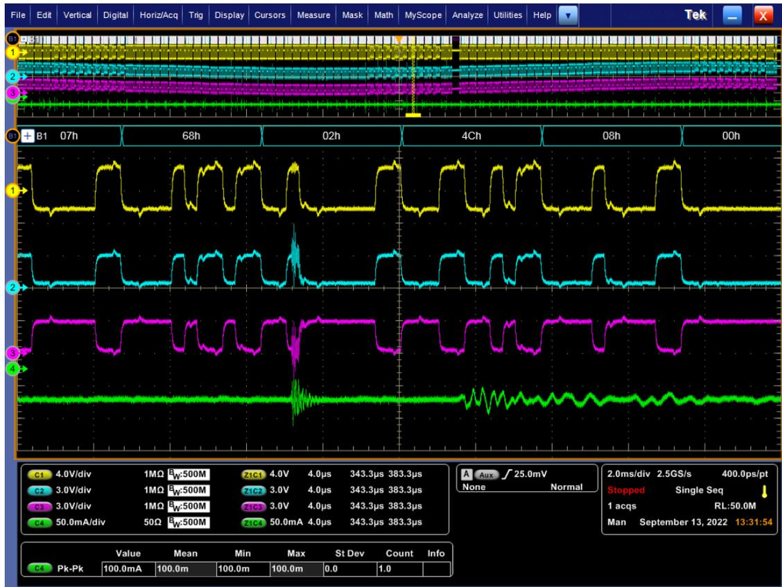
Figure 163: Ignitions on another segment (A2823) with Würth Elektronik DB9 with capacitor (measurement on segment A2825)
