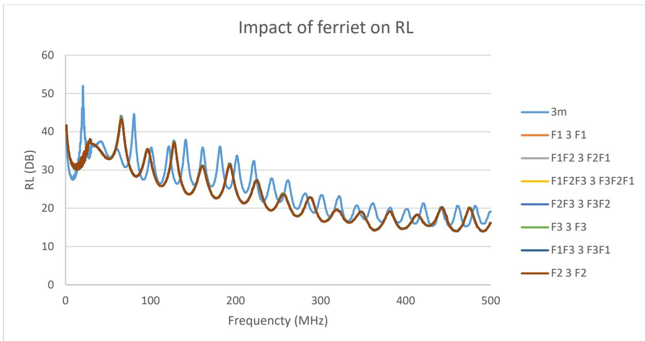
Figure 70: Impact of ferrite on RL
