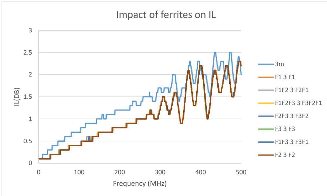
Figure 69: Impact of ferrite on IL
