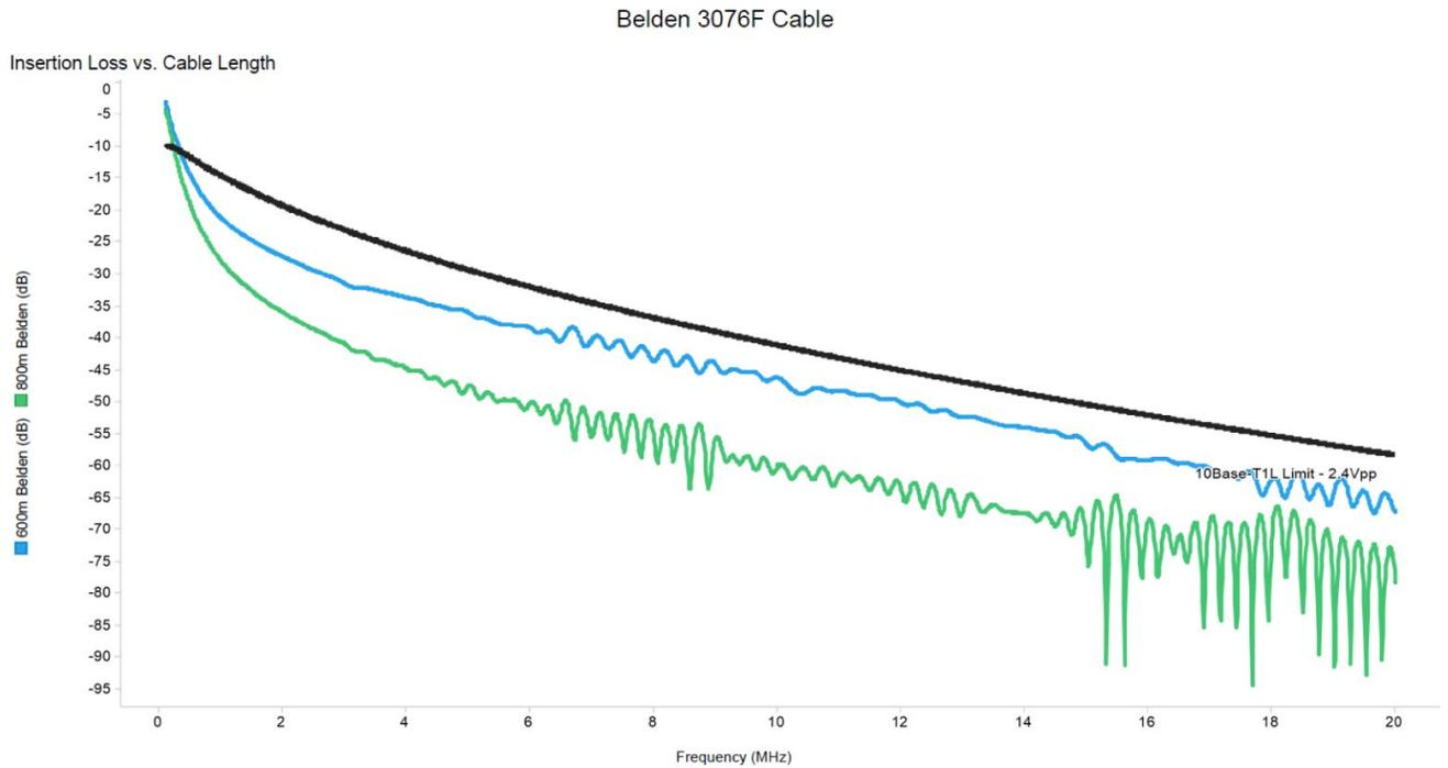
Figure 116: Texas Instruments measurement on Belden 3076F cable
