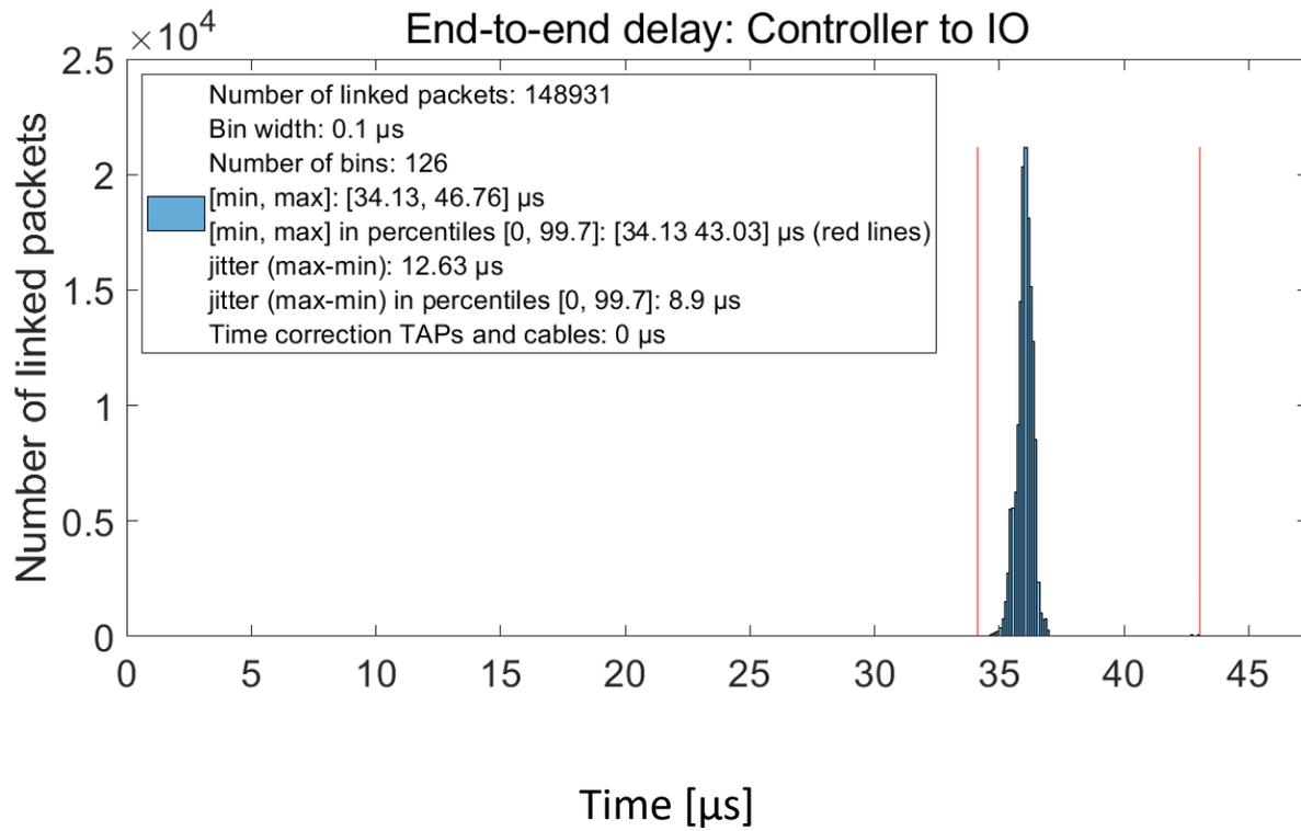
Figure 126: Phoenix Contact and NXP, 1000BASE-T, without preemption, without BE traffic
