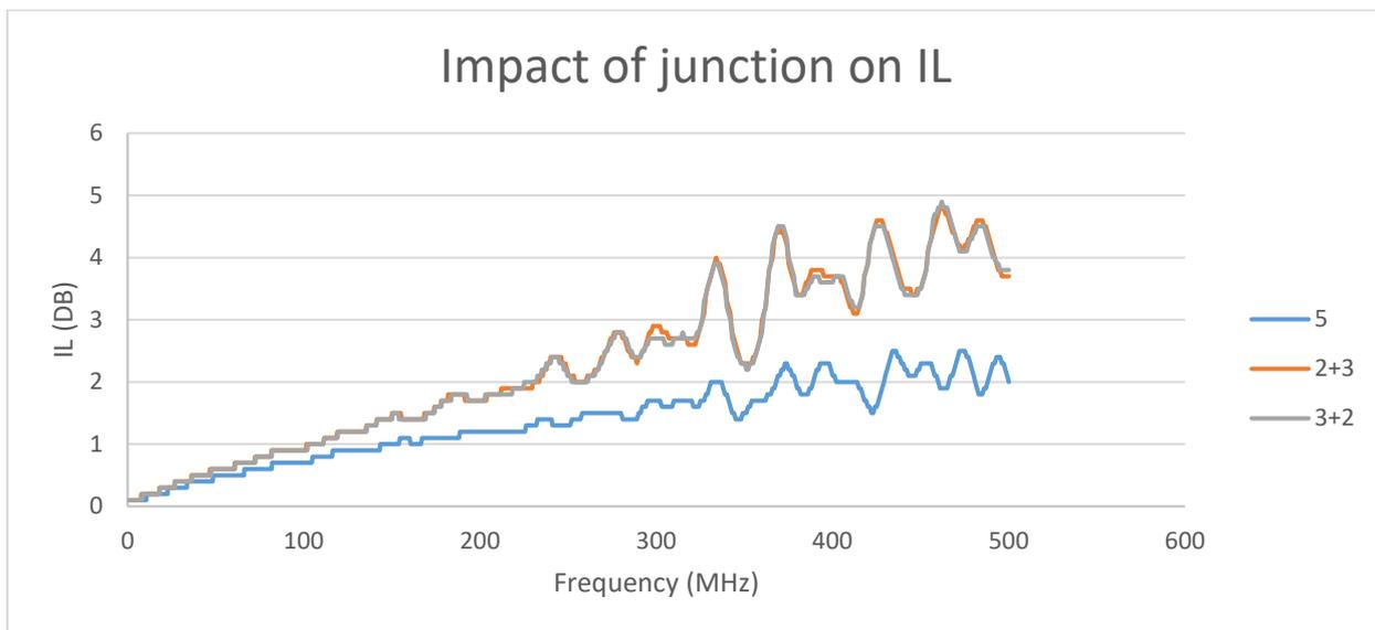
Figure 56: Impact of junction on IL on 5m cable
