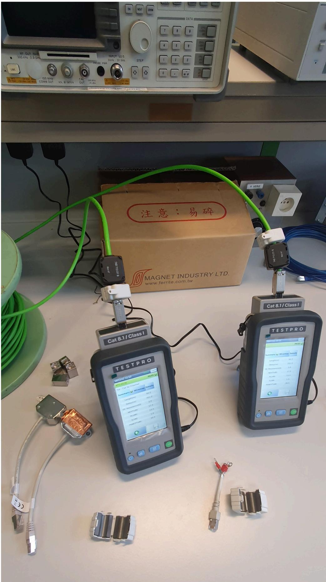
Figure 68: Experiment with 2 ferrites on each side
