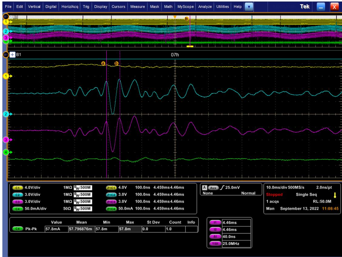
Figure 156: Ignitions with separate capacitor (segment A2825) (3)
