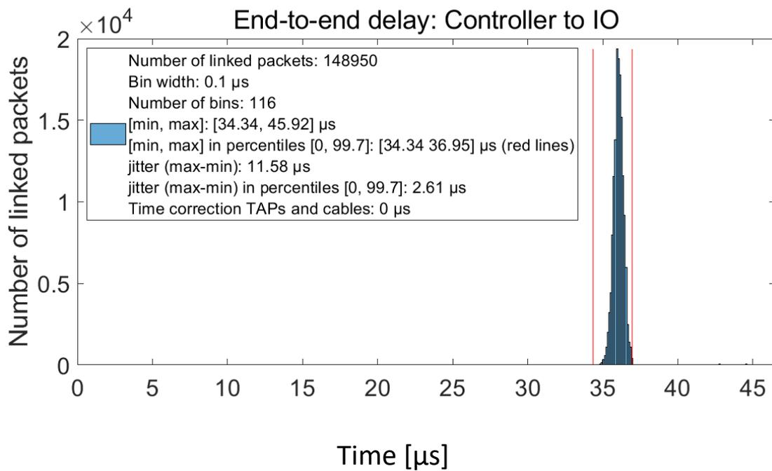
Figure 128: Phoenix Contact and NXP, 1000BASE-T, with preemption, without BE traffic
