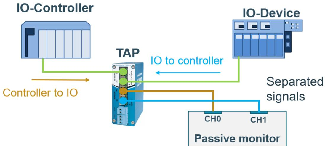
Figure 98: Connecting a TAP with passive monitor
