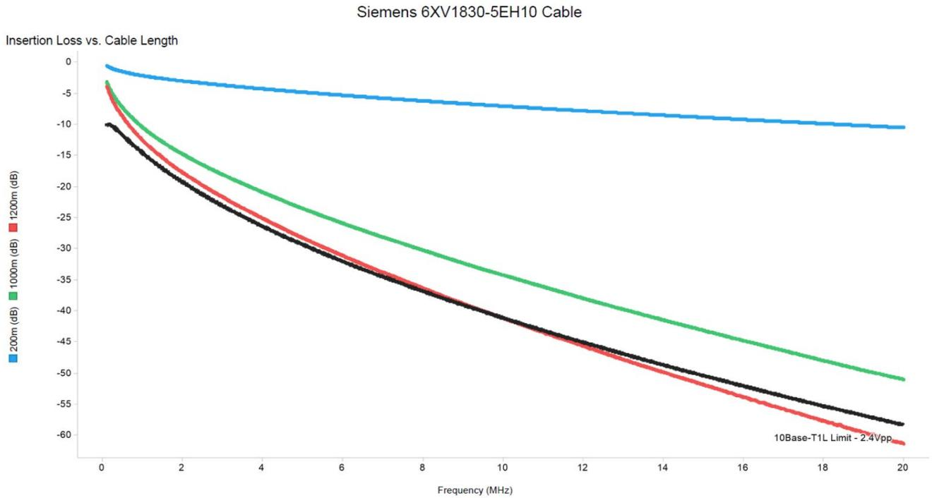
Figure 115: Texas Instruments measurement on Siemens 6XV1830-5EH10 cable
