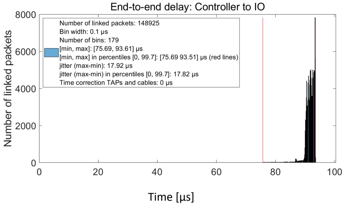
Figure 124: Relyum and NXP, 1000BASE-T, without preemption, with BE traffic
