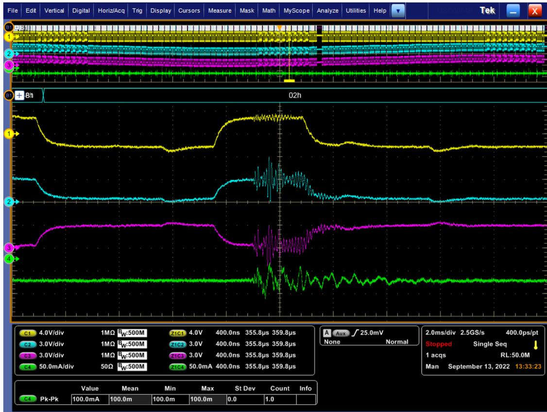
Figure 164: Ignitions on another segment (A2823) with Würth Elektronik DB9 with capacitor (measurement on segment A2825)
