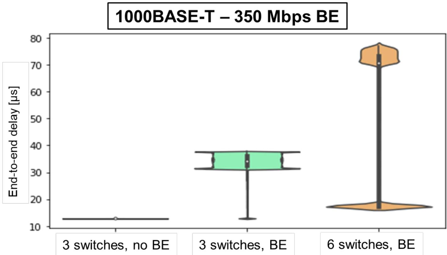
Figure 81: End-to-end delay on 1000BASE-T (350 Mbps BE)
