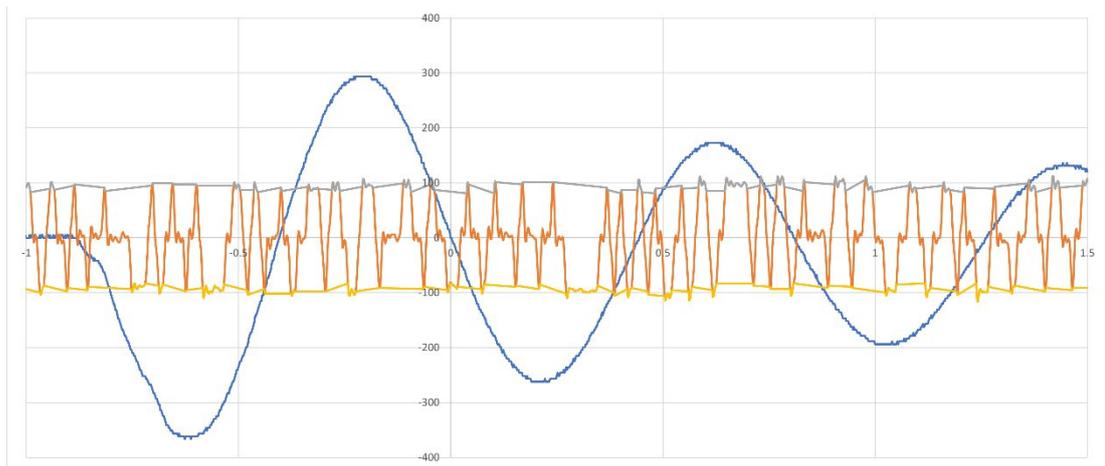
Figure 76. Shield current (blue) and PN communication (orange)
