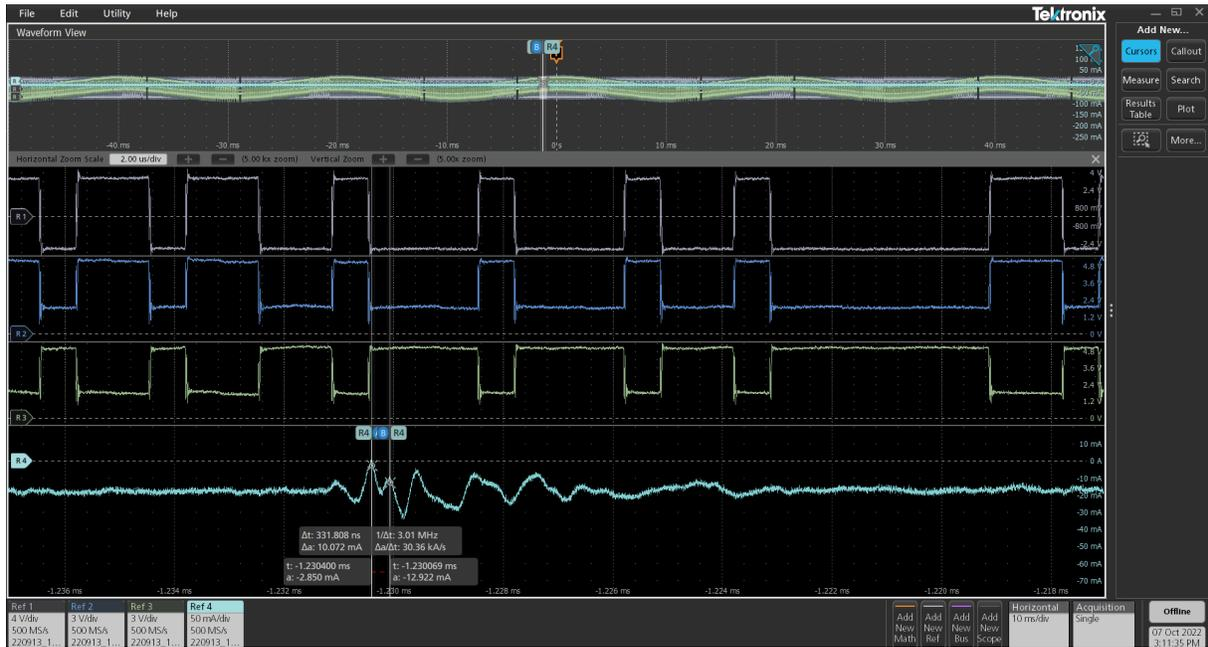
Figure 152: Zero measurement with loose capacitor no burner pulses (segment A2825) (4)
