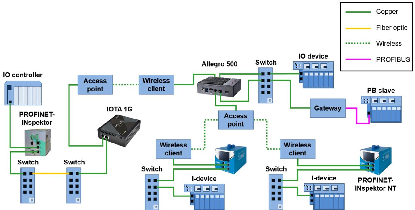
Figure 134: Overview of the measurement setup
